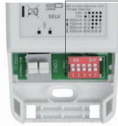
LED Current & Voltage Selection
