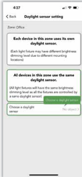
Figure 17.10 Choose a daylight sensor
